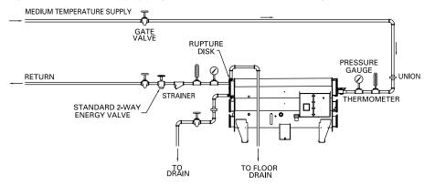
HOT WATER PIPING, 270 F AND BELOW VARIABLE FLOW THRU GENERATOR
